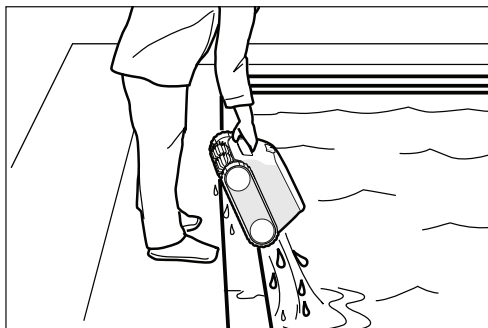
Figure 9. Keep Cleaner Vertical to Drain Water
